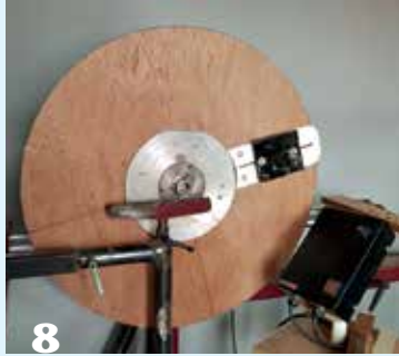
8 Back of carrier disk, showing mounted counterbalance unit (at right of disk). Workpiece is mounted on opposite side of disk, in line with counterbalance. Adjust the position of the metal weight until good rotational balance is achieved.
