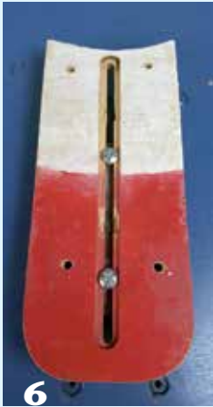
6 Front of counterbalance unit, with a countersunk groove.
