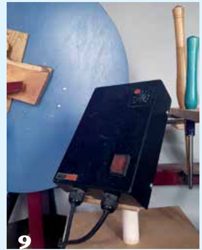
9 Ensure you can safely reach the lathe controls during turning. Never reach across or near the spinning workpiece/carrier disk. Reposition the controls as needed.
