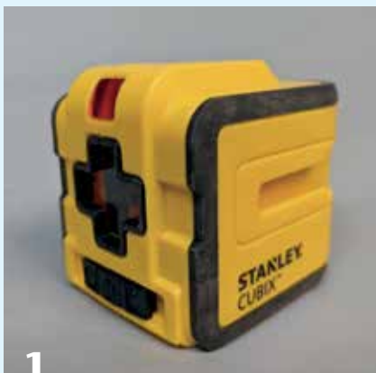
The author fitted a crosshairs laser to a camera monopod above the lathe bed, allowing the laser to be slid up and down as required. The closer the laser is to the workpiece, the finer the crosshairs.
