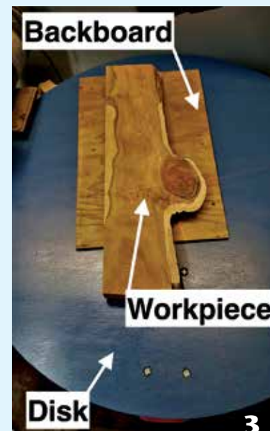
First, screw the backboard to the back of the workpiece, then screw the backboard to the carrier disk. Note the laser crosshairs aligning the intended turning center of the workpiece with the center of the disk.
